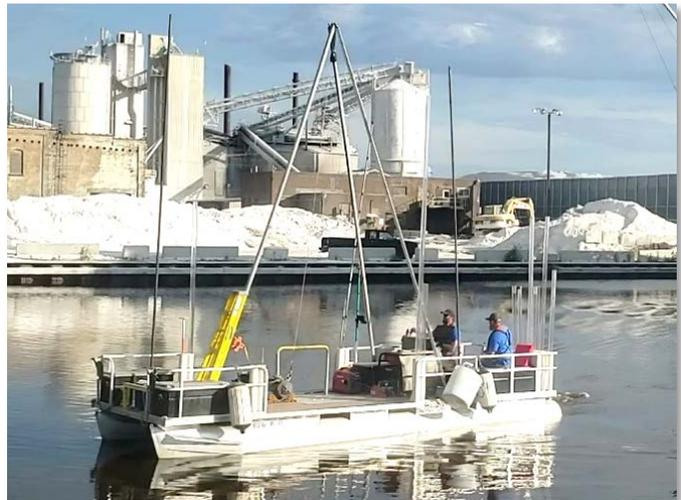
The 25' sediment sampling vessel also includes a depth-sounder, navigational GPS, 450W inverter, 2000W generator, VHF marine radio, 2 anchoring spuds for shallow-water stationing, and three *Danforth*-type anchors for stationing in deeper waters. This vibracore vessel is capable of collecting vibracore sediment core-samples up to 16' in length; in water depths as deep as 250' and in water depths as shallow as 2'.
